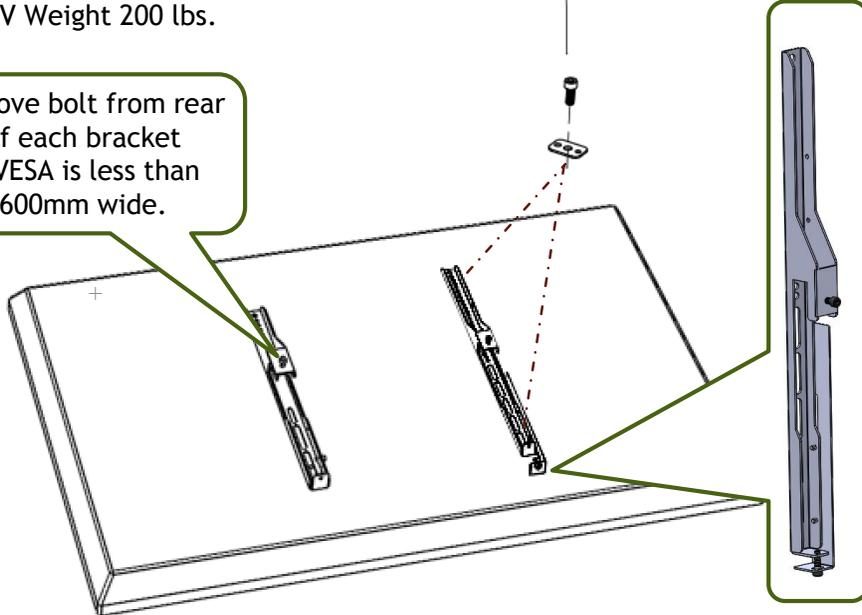
Uses Non-locking on left and locking bracket on right side.
